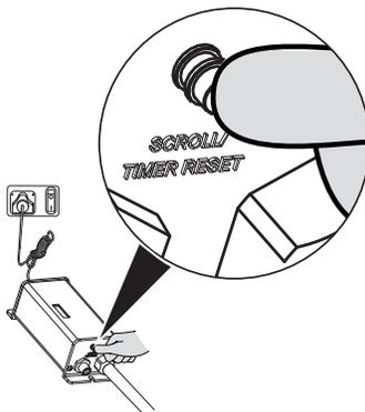
Hold down the timer reset button and reapply power to the controller until you see **RESET**, then release timer reset button. A 5 second delay will occur until you hear an audible tone and LED display will read once again **365**.
